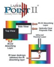
PCI offers a patented laser ablatable film for newer infra-red laser plate imagers with a vacuum system. It offers substantial cost savings in that you no longer need an image setter, just a laser (a \$25.000 -\$100,000 savings on equipment, not to mention ongoing maintenance and precious metal films), further the process is chemical free. Since the product is competitively priced, the consumer
